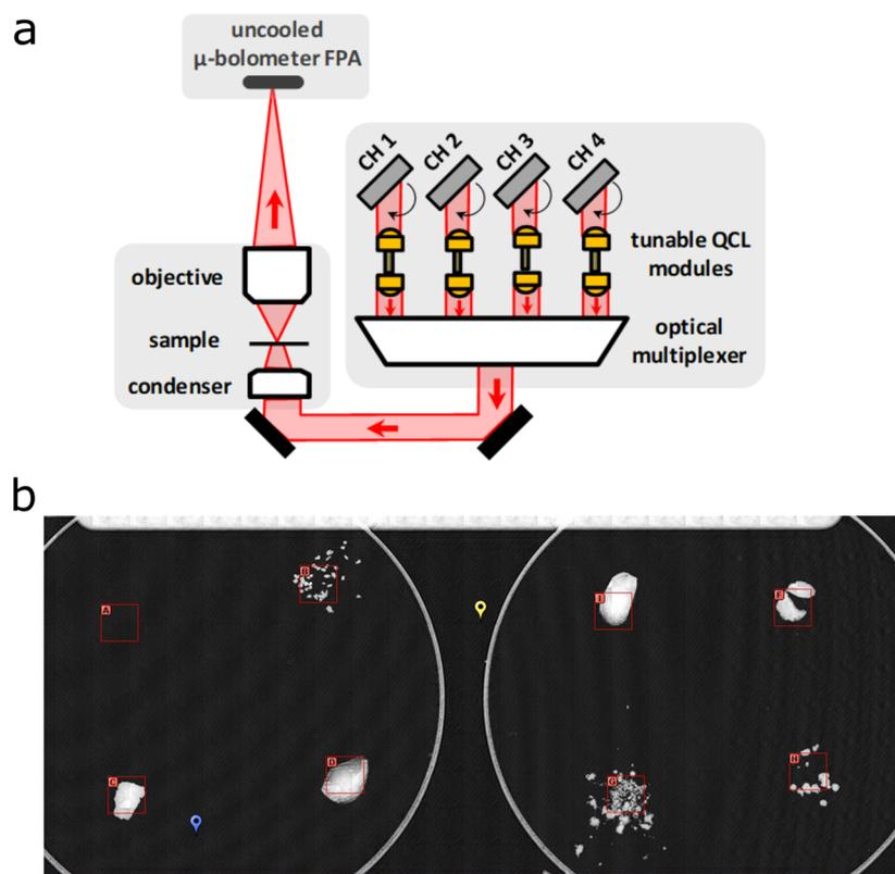
**Figure 1.** (a) Schematic overview of the beam path in the microscope from the quantum cascade laser (QCL) setup containing four laser chips (CH1 to CH4) measuring the sample in transmission before reaching the micro ( $\mu$ ) bolometer focal plane array (FPA) detector. (b) False-color image at  $1470\text{ cm}^{-1}$  of the sample stage with reference materials placed on barium fluoride ( $\text{BaF}_2$ ) windows ( $d = 25\text{ mm}$ ) with selected (red squares) measurement fields.
