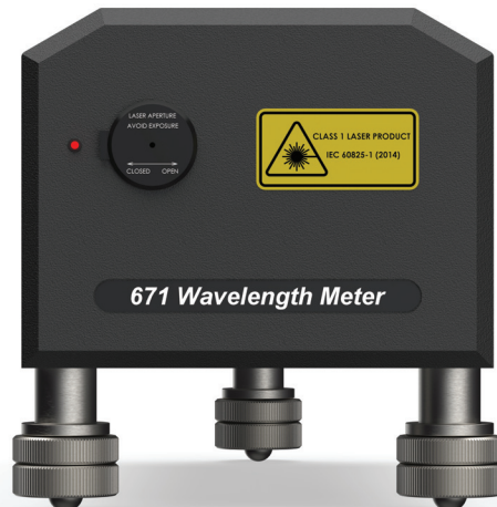
Figure 6. Front panel layout for free-space models. (Note: aperture and height adjustable legs)
