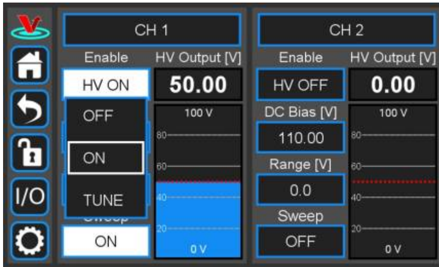
Fig. 20: Controlling the internal ramp
