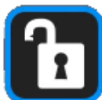
Fig. 7: Lock button (shown in unlocked mode) Locks out further modification of operation parameters. Touch to lock or unlock parameter entry. When in lock mode, it is still possible to toggle the ramp on and off, but it will not be possible to turn on the high voltage, change the bias voltage, or edit other operation parameters.
